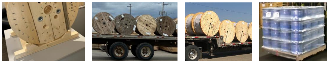
Figure 5 – Packaging methods (from left to right): Cradling, Chocking/Blocking, Strapping, and Palletizing
